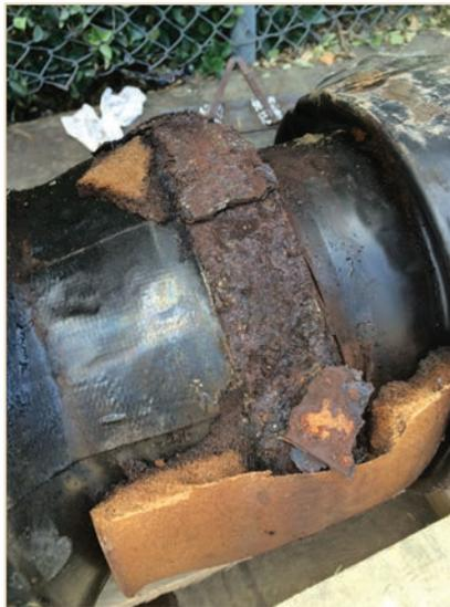
PHOTO 1 Ductile iron pipe joint corrosion (18 years).
