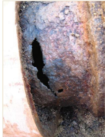
PHOTO 2 Ductile iron pipe joint failure (10 years).
