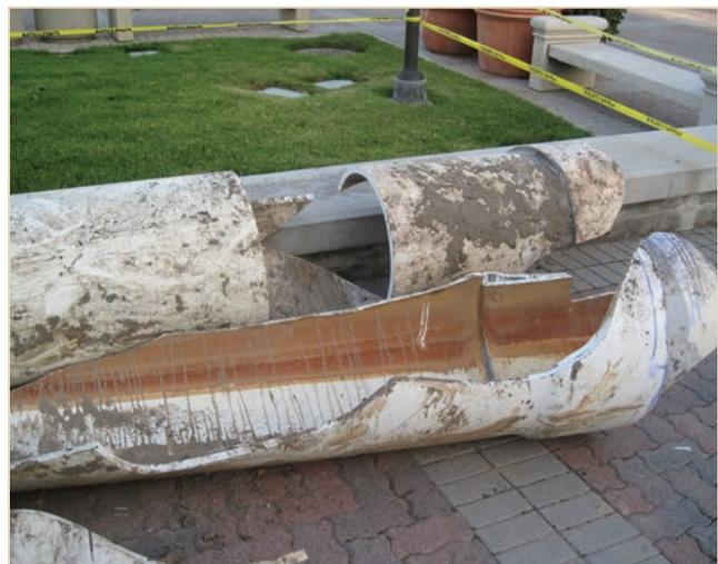
PHOTO 3 SDR 26 PVC pipe failure (22 years).
